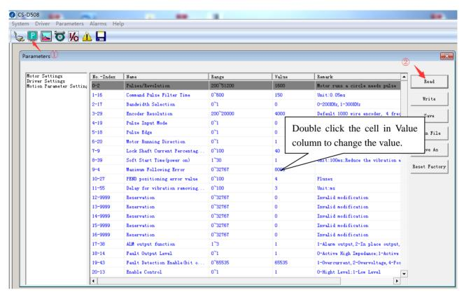
The parameter classification in the left of the ProTuner is available when using vector easy servo of ES-D508-V, ES-D1008-V, ES2-DA808 and ES2-DA1208. Because the two series drives use the one same ProTuner.
