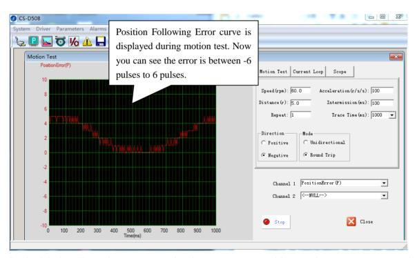
In the Motion Test tab, you can make the motor rotate without pulse generator or motion controller. Configure the trapezoid velocity file first and then click the **Start** button. There are two channels can be used to monitor the "Current Feedback, Position Error, Position Feedback, etc." as below:
