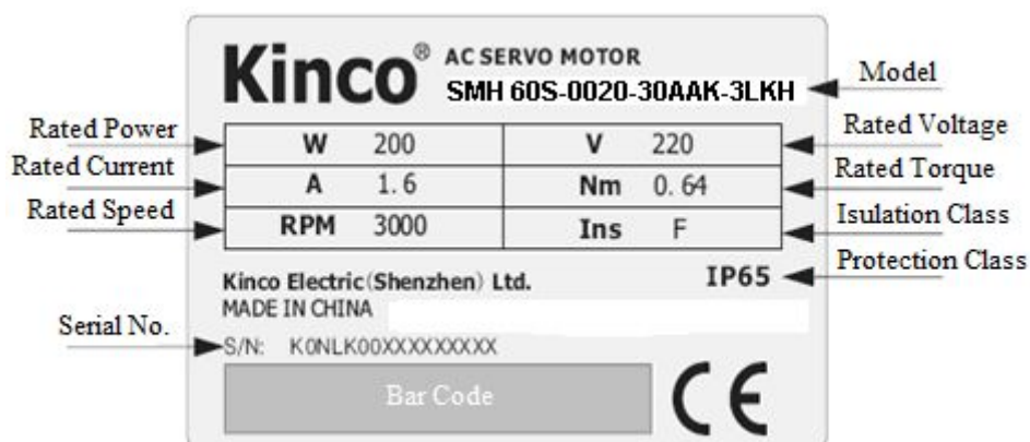
Fig. 1-2 Nameplate of a servo motor
