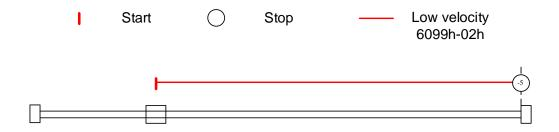
Mode -4: Search for homing point in negative direction at high velocity. Move in positive direction after torque reaches the value set in Pr5.39, stops when torque is gone. Homing done signal delivers after the time value set in Pr5.37
