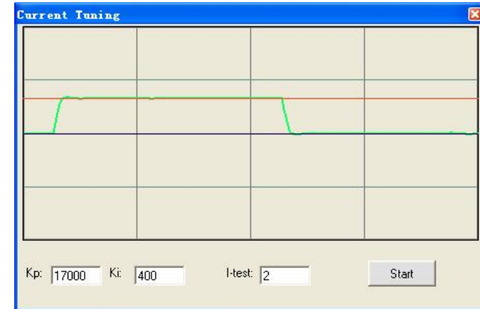
Figure 29: Step response with better K_p and K_i of current-loop ( K_p=17000, K_i=400 )
