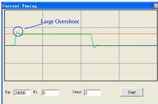
Figure 28: Response with High K_p of current-loop ( K_p = 24000 )
