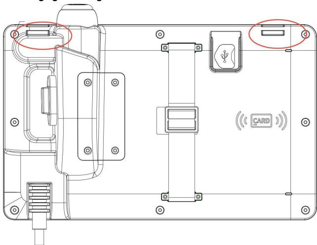
The top is reserved for the strap design, and the 600\*20mm black nylon braided lanyard is used through the upper two holes reserved at the left and right ends of the top of the back shell. Hung in the ideal position for control.
