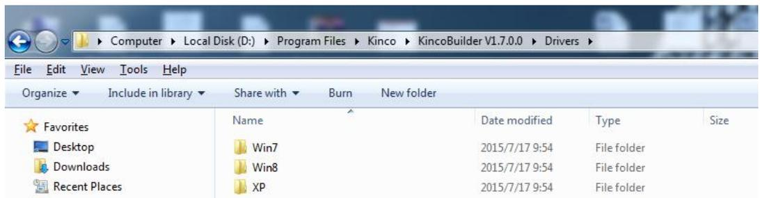
When connecting programming cable to MK series and PC first time, Windows system will detect new hardware and mention installing driver, users can install the driver according to the version of Windows.
