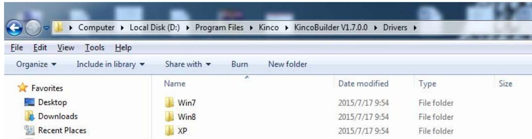
When connecting programming cable to HMI-PLC and PC first time, Windows system will detect new hardware and mention installing driver, users can install the driver according to the version of Windows.
