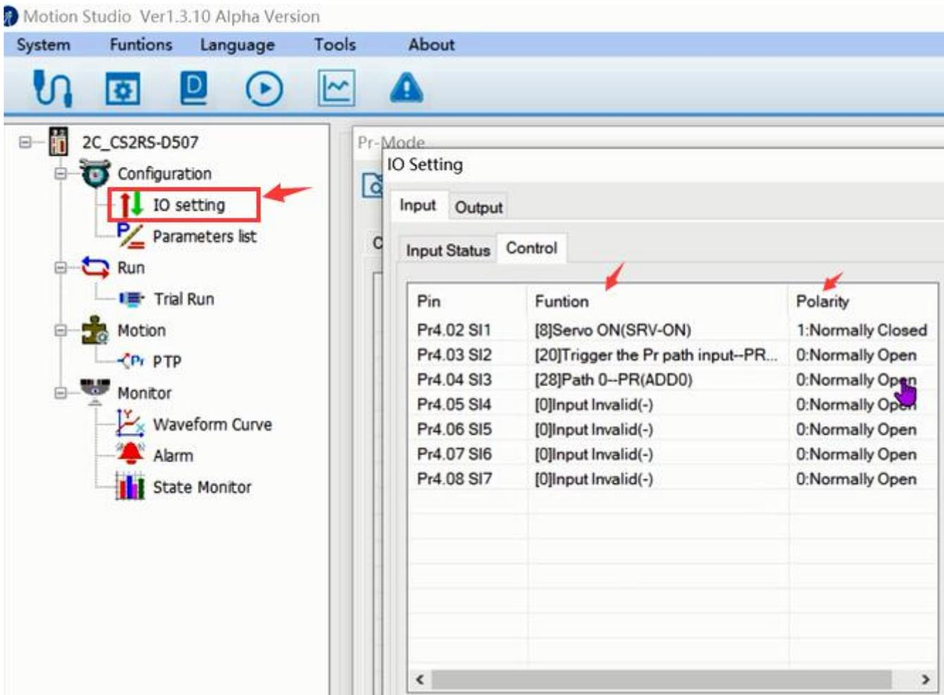
*Note: After setting the parameters, click "OK". Then, in the parameter management window, click the Save button to prevent the parameter values from being lost after the drive is powered off.*
