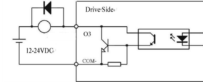
**Figure 3.4: Output Interface Wiring**
