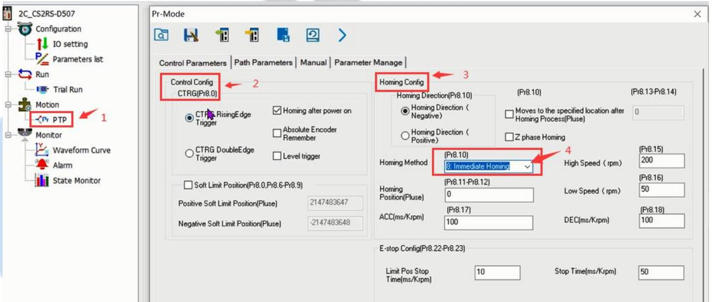
(2) This window is the PR path parameter setting, including operation mode, target position, speed value, etc. Double click to modify parameters.
