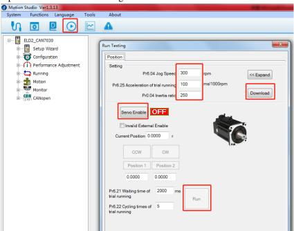
1. Before starting the "Run", you need to set the relevant objects for the movement itself like "jog Speed", "acceleration of trial running", "inertia ratio" and "Expand".
