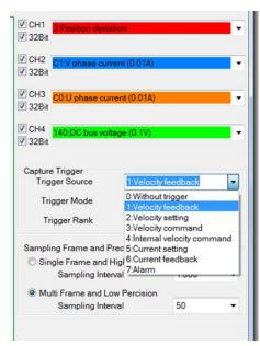
2. Click the button "Capture", you can monitor the status of performance when the motor is running. For example, the driver and motor are running position feedback position error velocity feedback and current feedback.
