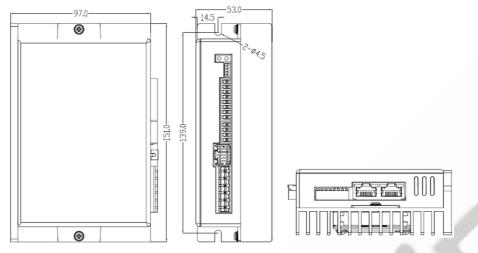
CS2RS-D1008 Figure 2.1: CS2RS series mechanical drawing
