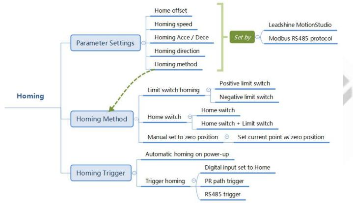
Zero Position: a fixed position on the machine can correspond to a definite digital input signal, or to a Z signal Zero Point of Machine: mechanical absolute zero position
