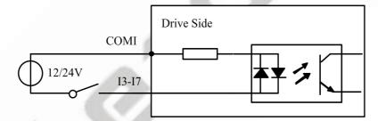
COMI: can be connected to 12 / 24 V (common-anode), or 0 V (common-cathe
