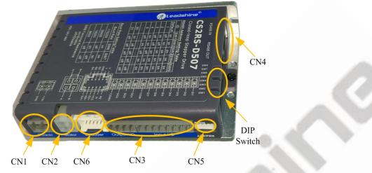
Figure 3.2: CS2RS series connectors
